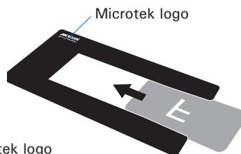
3. Load and insert the 8.5" x 4.5" Film Holder with loaded film into the Feed Tray, with the side to be scanned facing down and with the top of the film directing downwardly.
