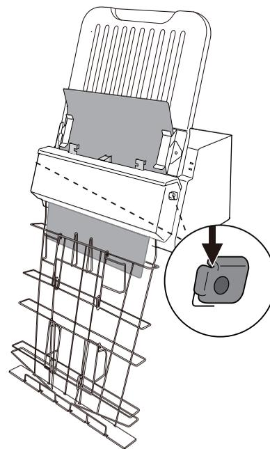
2. After opening the front cover, let the jammed film fall into the output basket and then remove it from the output basket.
