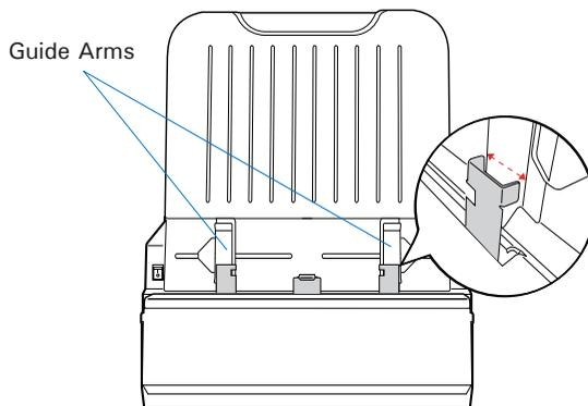
3. Push down the Light Shield. Make sure that two fastenings of the Light Shield are attached to protruding parts at the bottoms of Guide Arms tightly. If the Light Shield and Guide Arms are jointed successfully, they can be moved together by sliding Guide Arms.
