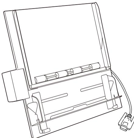
The coming section describes how to install the AFF on the MII-900 Plus through the MII-900 Plus's accessory port and how to scan X-ray films by using the AFF.
