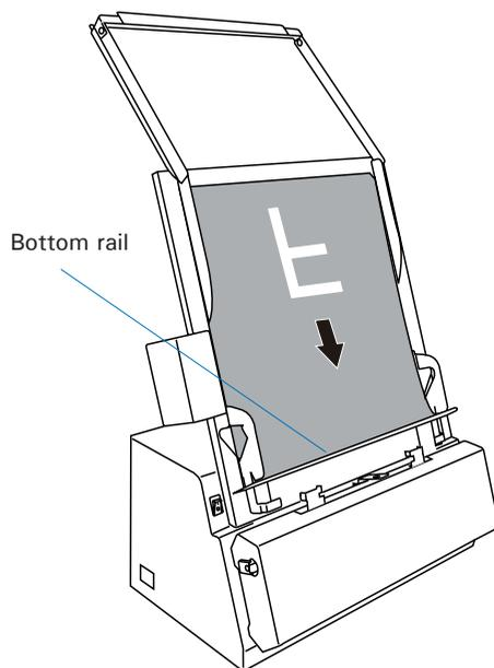
Please take note that the bottom of the films should be placed against the front side of the bottom rail as shown in the graphic and rest the back against the AFF housing.
