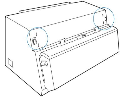
2. Insert and push down both sides of the Feed Tray into its compartment holes, making sure the Feed Tray snaps into place.
