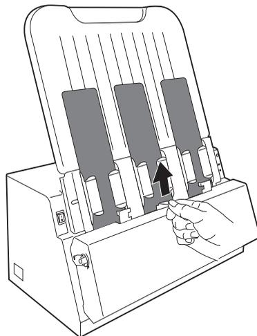
**NOTE:** If you would like to scan less than 3 sheets of X-ray films at a time, make sure that you have to put one sheet of X-ray films at the middle channel. For example, when scanning two sheets of X-ray films, you should put the first one sheet of X-ray films at the middle channel. Then, you can put the other one at either the left or right channel as preferred.
