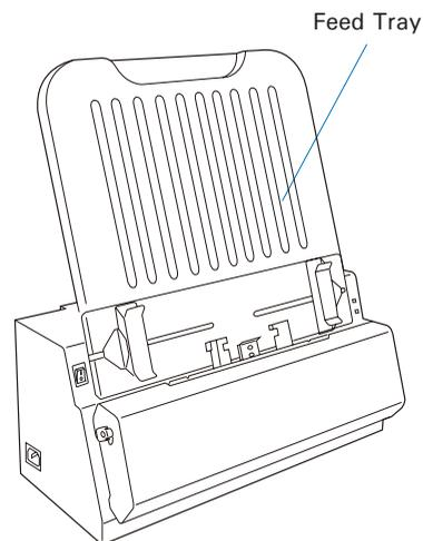
2. Load and insert the film into the Feed Tray, with the side to be scanned facing down and with the top of the film directing downwardly.
