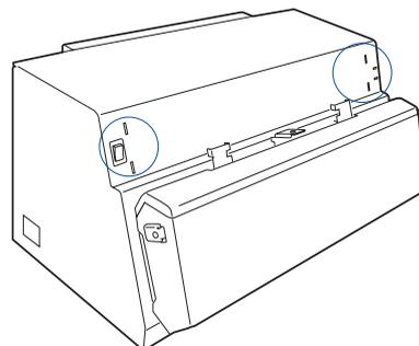
2. Insert and push down both sides of the AFF into its compartment holes, making sure the AFF snaps into place.
