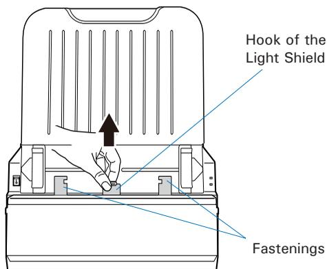
2. Slide the two Guide Arms toward the Light Shield. Align the Guide Arms with the fastenings of Light Shield properly.
