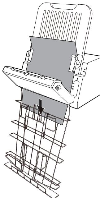
**NOTE:** To remove the jammed film from the digitizer, you have to open the front cover first. Otherwise, your film may be damaged if they are forcedly removed.
