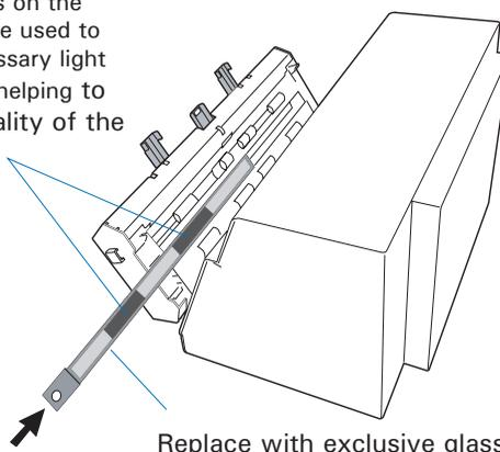
**NOTE:** Make sure that the exclusive glass for the Multi-Channel tray is fully inserted and snapped into place.
