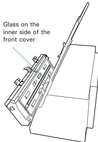
2. Find a perforation at the left of the glass. Use it to pull out the glass, shown as in the graph below.
