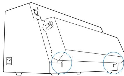
2. Insert and push down both sides of the Output Guide into its compartment holes (a), making sure the Output Guide snaps into place.
