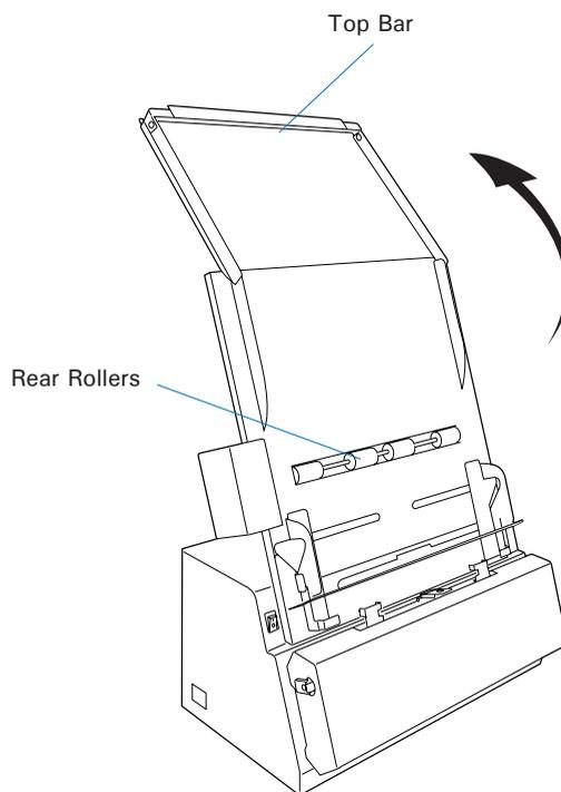
3. Load the films into the AFF Tray, with the side to be scanned facing down and with the top of the film directing downwardly.
