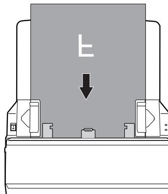
4. Align the film with the center of the Feed Tray by sliding the two Guide Arms toward the film if the width of the film is less than 14" (35.56 cm)
