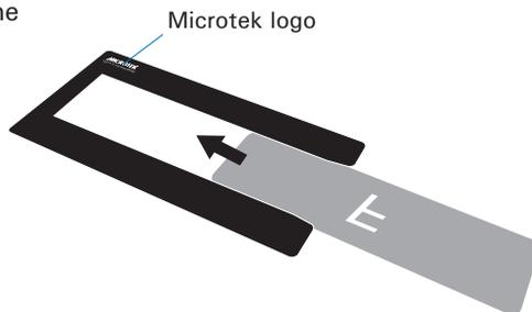
3. Load and insert the 12" x 3 1/3" Film Holder with loaded film into the Feed Tray, with the side to be scanned facing down and with the top of the film directing downwardly.
