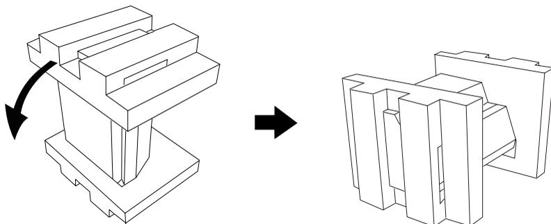
4. With both hands, hold the two sides of the digitizer with the foam supports attached, and then put the digitizer back into the shipping carton.
