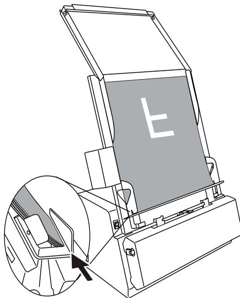
4. Lower down the Top Bar onto the films so the films are sandwiched between the Top Bar and the AFF tray.
