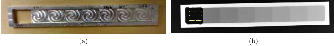
Figure 2. (a) Picture image of the Step-wedge and (b) Exposure image of the step-wedge
