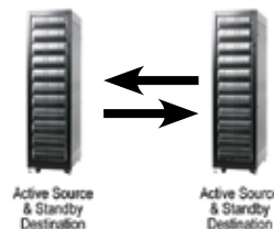
Failover Bi-Directional Data Replication
